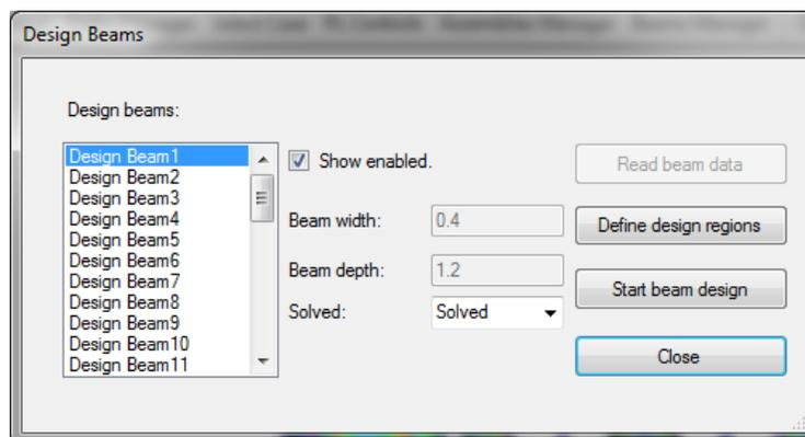
After loading the beams, the beam breaks and design sections positions can be defined using the “Define design regions” button. This menu allows the user to define and/or modify break and section positions using their relative or absolute position simultaneously.
