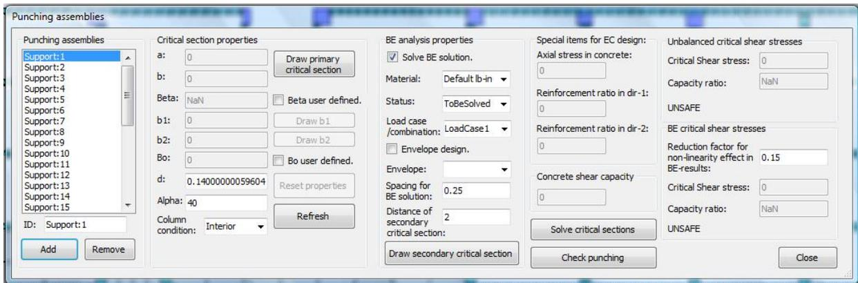
The variables defines in the critical section properties window are similar to punching critical section properties as stated by ACI-318.
