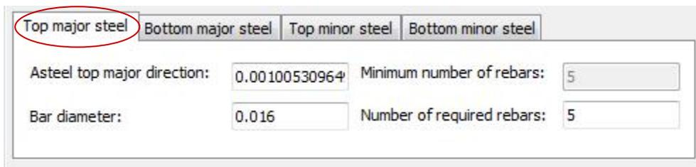
Choose the Bar Diameter, the corresponding minimum number of rebar will show up, thus input the integer number of required rebar.
