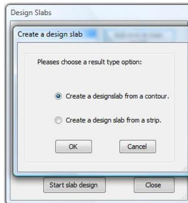
If you choose to create design slabs from contours, you will reach this menu that can be used to create multiple design slabs from local contours.
