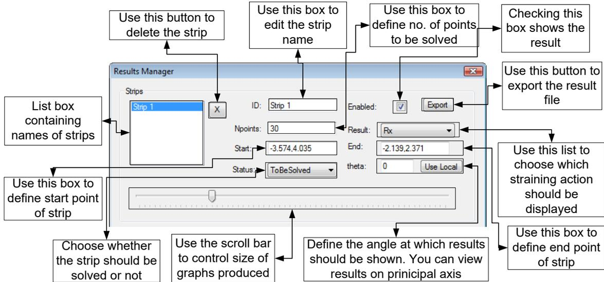
Strips: This part of results manager is used to control strip properties including ID, Start and End points, No. of points within the strip, type of stress resultant that is required to be displayed at this strip. Export command is used to export a tabulated format of the strip results, the produced tables can be used by any spreadsheet software.
