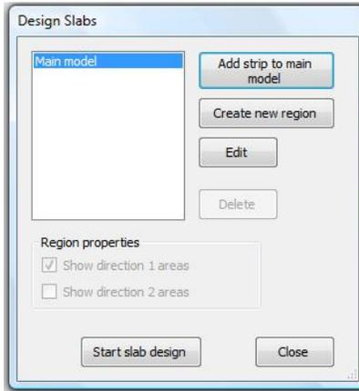
Press on “Start slab design” to start showing the as required for each design slab in both X and Y directions.
