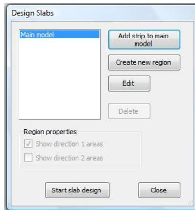
When you choose to “Add strip to main model” a design slab, this dialogue box will allow you to create design slabs from ready local contours or strip results (present in the Results Manager).
