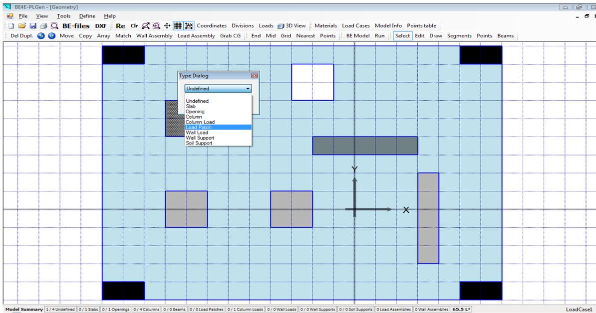
To define the load properties, Right Click on the column without choosing it by Left Click. Use the produced dialogue to define the loads induced at this patch which is a uniformly distributed load. This window allows you to define the number of boundary divisions in X and Y direction.
