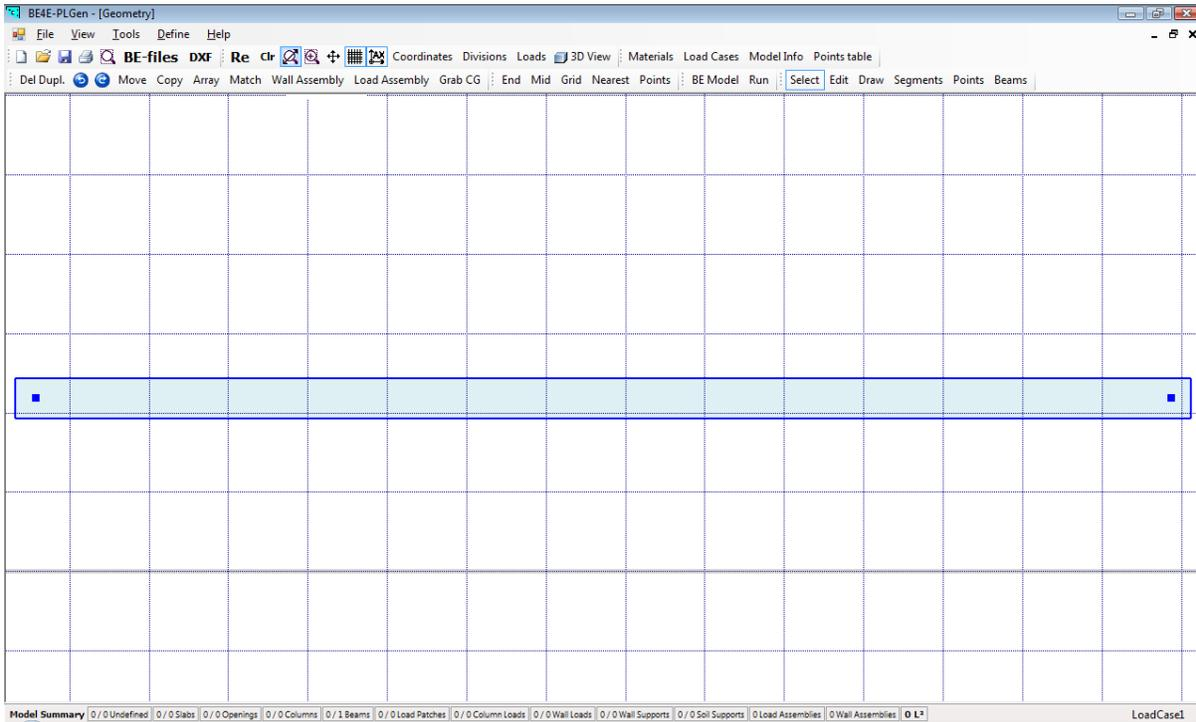
To define the beam properties, Right Click on the beam without choosing it by Left Click. Use the produced dialogue to define beam depth, width, start point, end point, moment of inertial ( $I_y$ ), Torsional constant ( $J$ ), material, number of divisions, defining own weight per unit length of beam and whether the PL should include the beam own weight or not.
