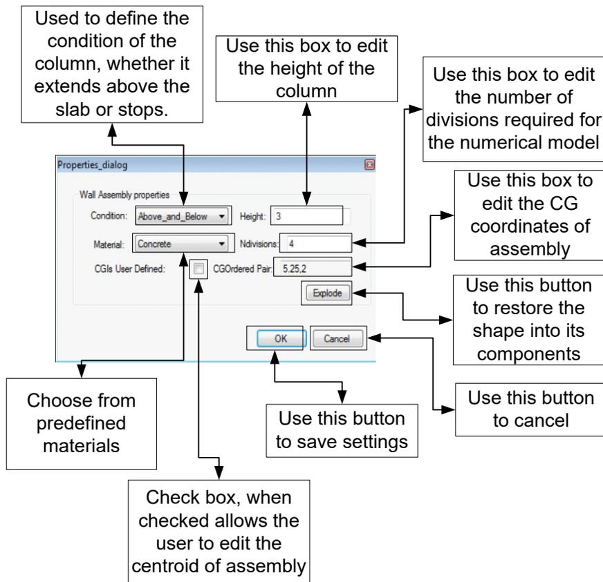
By right clicking on the produced shape, the above dialogue box will appear which is used to define the properties of the wall assembly produced. Using the wall assembly, the PL calculates the new position of the CG of the assembly and hence calculates the inertia and stiffness accordingly. The Explode button divides the assembly into its original components.
