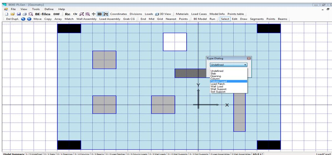
To define the column properties, Right Click on the column without choosing it by Left Click. Use the produced dialogue to define the loads induced by this column. The load has three parameters vertical force (F), moment in X direction (Mx) and a moment in Y direction (My).
