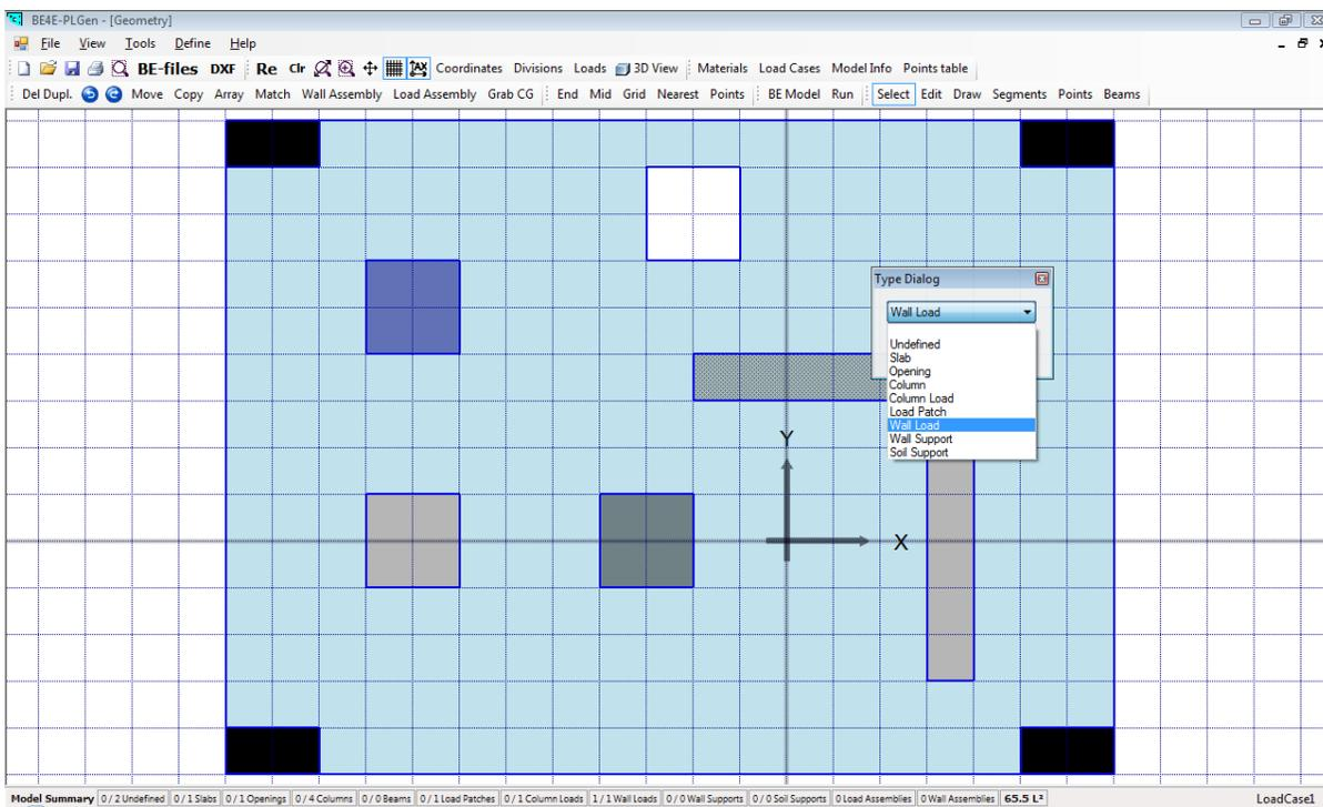
To define the wall load properties, Right Click on the wall without choosing it by Left Click. Use the produced dialogue to define the loads induced by this wall. The load has three parameters vertical force (F), moment in X direction (Mx) and a moment in Y direction (My).
