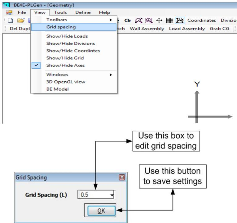
Brings up a small window allowing the user to choose the grid spacing on the screen, PL grids are square.
